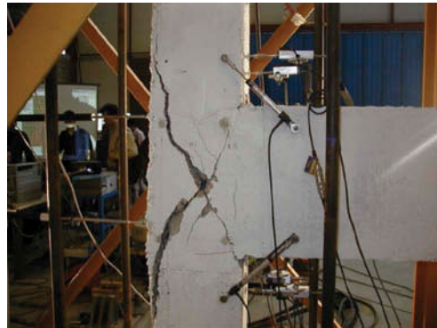
(b) Diagonal cracking in joint.
